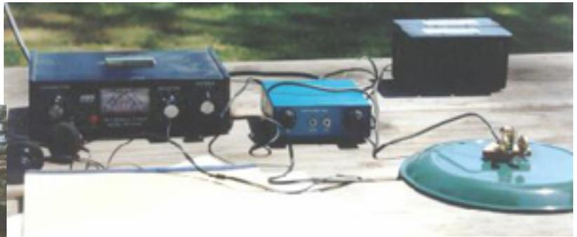
Tuner, QRP Radio and Key
