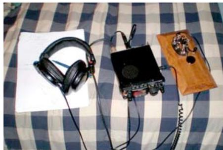
Donald's Straight Key Night set up was a very minimal affair consisting of a straight key, headphones, a Yaesu FT-817ND all-band QRP transceiver, a NorCal Balanced Line Tuner (BLT) and a homebrew 88' doublet that included homebrew ladder line and a water bottle top center insulator.
