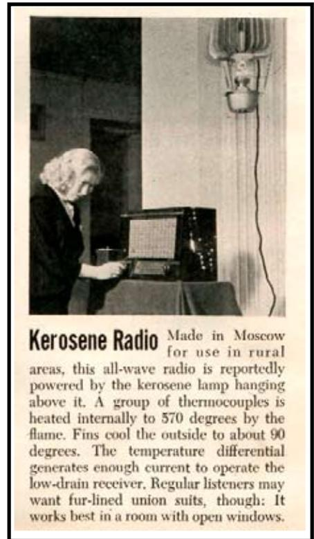
**Kerosene Radio** Made in Moscow for use in rural areas, this all-wave radio is reportedly powered by the kerosene lamp hanging above it. A group of thermocouples is heated internally to 570 degrees by the flame. Fins cool the outside to about 90 degrees. The temperature differential generates enough current to operate the low-drain receiver. Regular listeners may want fur-lined union suits, though: It works best in a room with open windows.
