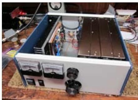
Something borrowed is this capacitor checker from the Heathkit era and like the AR88 it has maintained its value and usefulness. I was sceptical of some rather small electrolytics rated at 500 V and wanted some reassurance that they would be reliable. In a matter of seconds this tester showed that indeed the cap was happy at 500 V (but not at 600 V) and indeed had a value of 4 uF as marked. Not something one needs every day so great to have access to one.
