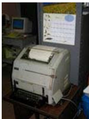
During my earlier days I operated CW on the national police net. We sometimes copied incoming messages directly to a Teletype keyboard, instead of a typewriter. A dedicated line connected with the remote destination terminal. The maritime stations were also connected with their customers via TTY and TWX connections.
