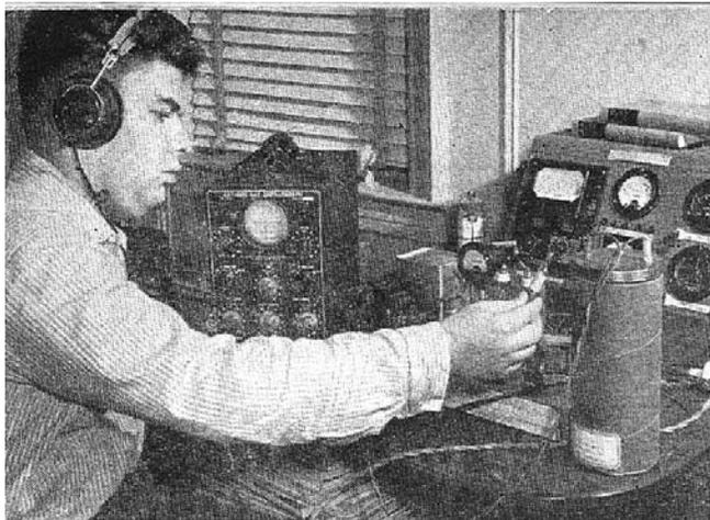
In his instrument-filled bedroom, Fishman shows how his homemade Geiger-Muller counter (right) registers nuclear particles. Rays from radium solution in tube show on oscilloscope at left.
