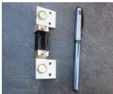
A 375 micro-Ohm 200 Amp current shunt
